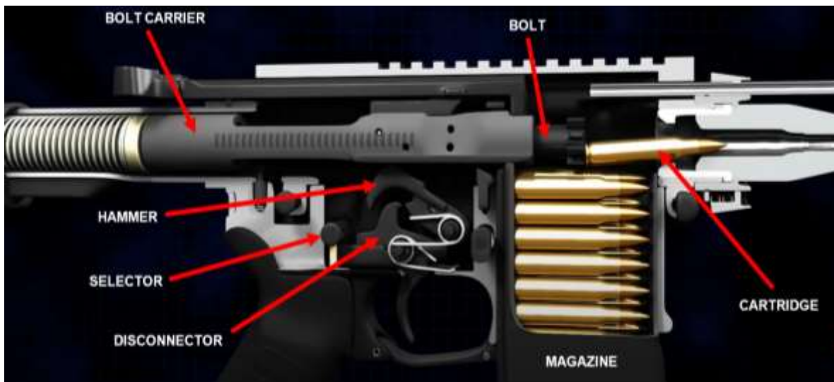
Figure 2: Post-fire forward motion of bolt carrier 4
