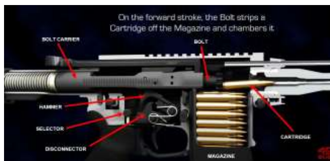
Figure 2: Post-fire forward motion of bolt carrier 4
