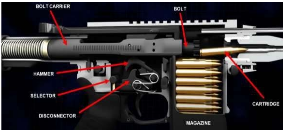
Figure 2: Post-fire forward motion of bolt carrier 4
