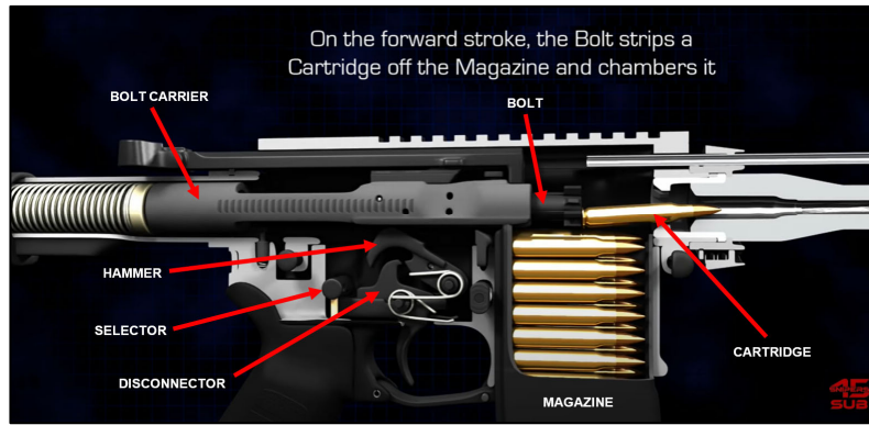
Figure 2: Post-Fire Forward Motion of Bolt Carrier 9
