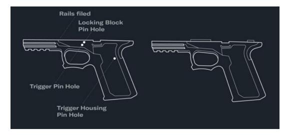
As is evident, the difference between the two frames is minimal. The functional frame contains three drilled holes (the locking block pin hole, the trigger pin hole, and the trigger housing pin hole), and the rails filed off. By adding these simple features to the unfinished frame with common household tools, any individual can make the unfinished frame functional in hours or less. *See* PI Amici Curiae Br. at 20-21.
