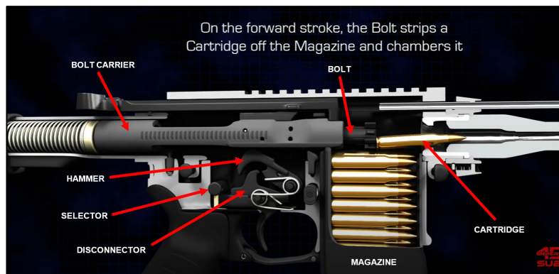
Figure 2: Post-Fire Forward Motion of Bolt Carrier 9
