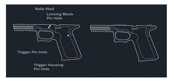
As is evident, the difference between the two frames is minimal. The functional frame contains three drilled holes (the locking block pin hole, the
